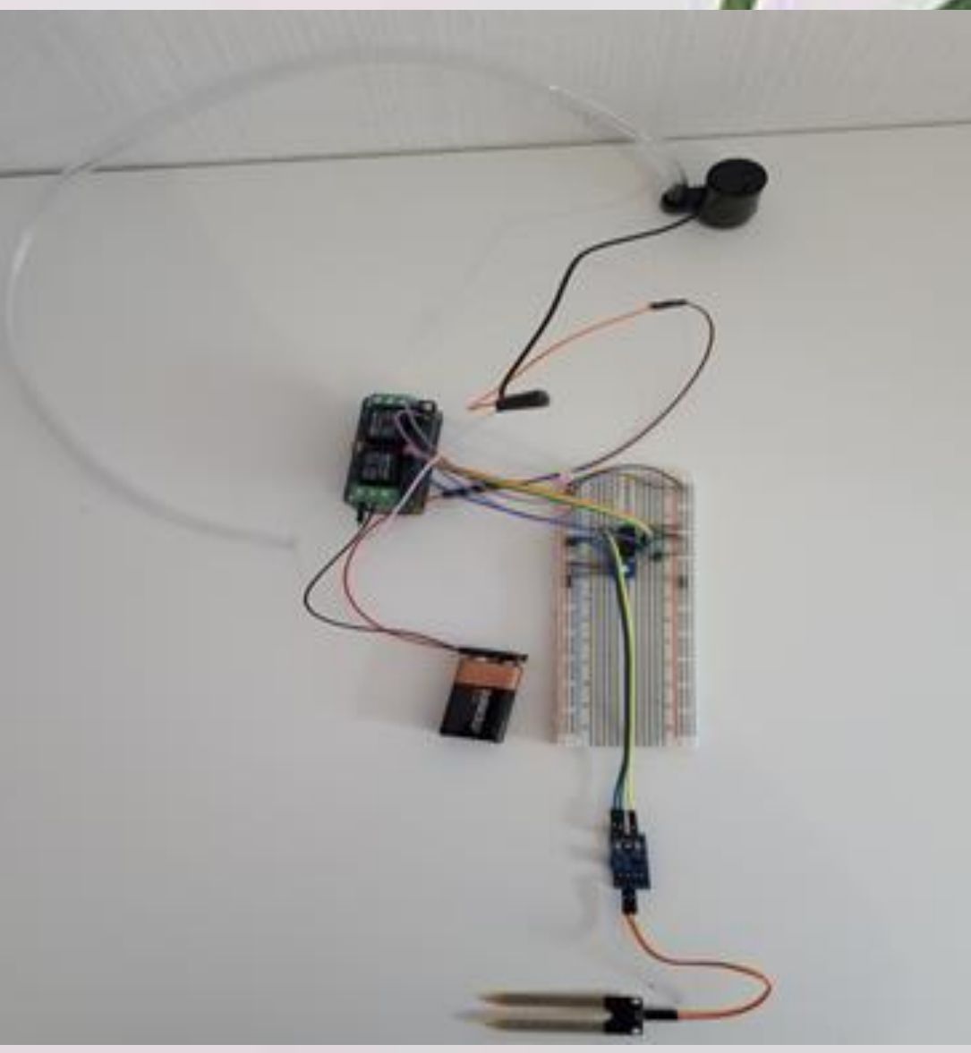
Figure 1: Fully Connected Plant Watering System
