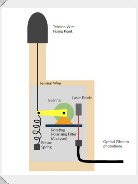
The input phase works by using the linear extension of a finger when bending to rotate a polarising filter with the attached gearing.
