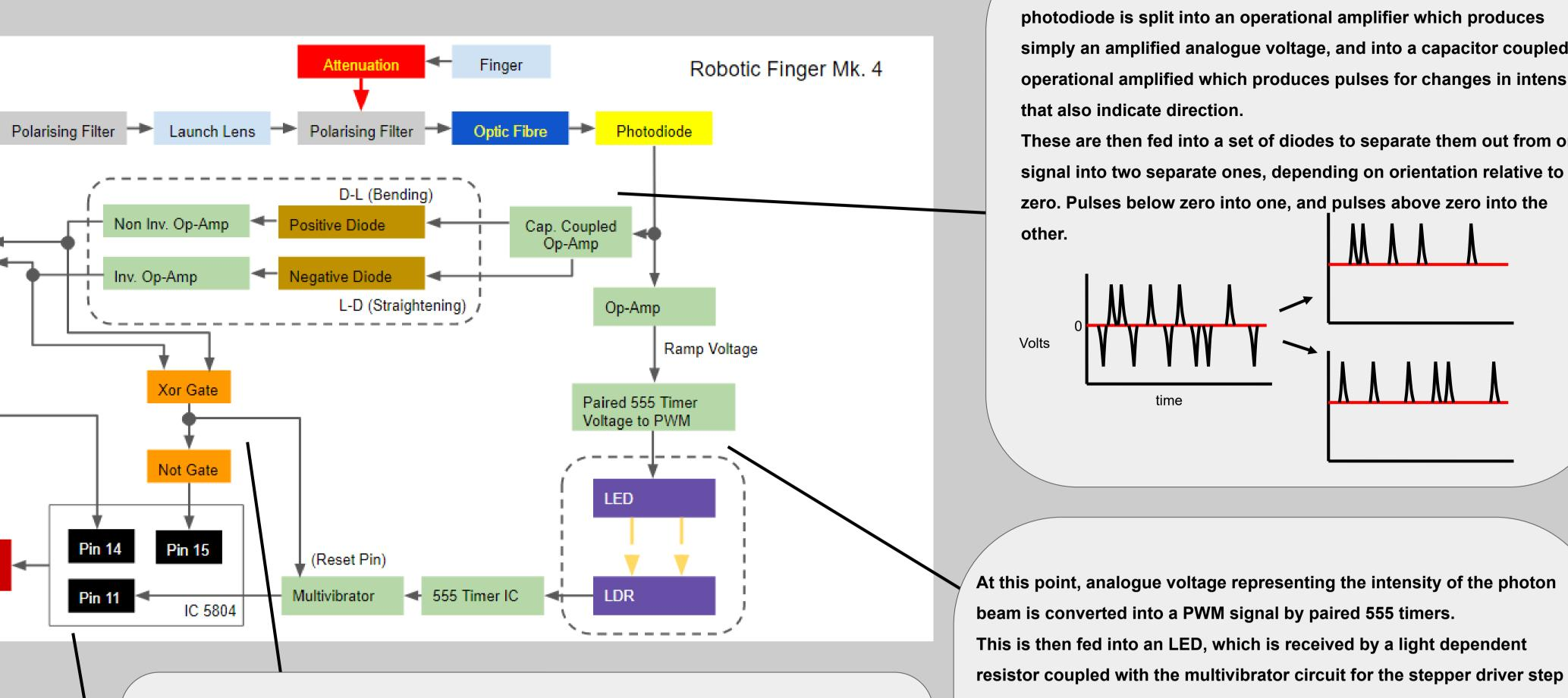
Here, both pulsed signals indicating changes in intensity are entered into an xor gate. The xor gate will determine if either of them are active (on). If neither are on, the interrupts for both the multivibrator and the stepper motor driver will be engaged and they will stop until they are required again.
