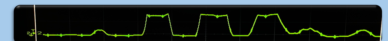
Figure 4. Output of Inverting Op-Amp
